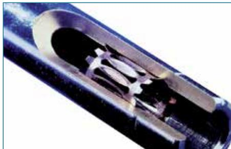
*The plugs and sockets have been provided with a self-cleaning system. An elastic shutter type spring casing has been installed in the inserting sleeve of the socket which ensures low contact resistance and low temperature rise while reducing the inserting and pulling-out force.*
