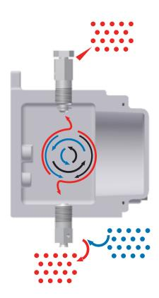
The sole installation of valve at the bottom with the combined function of drain and breather is giving, anyway, a good result and since the water penetration is practically impossible due to installation point, the IP66 protection is guaranteed also with the UVD model (always open).
