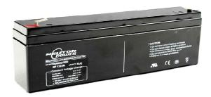
Neuton Power NP series are designed with AGM (Absorbent Glass Mat) technology and for general-purpose applications, such as UPS, telecom, and electrical utilities. These batteries are comply to most popular international standards, such as IEC60896-21/22, BS6290-4, Eurobat Guide. The battery container and cover are available both in V0 class flame retardant ABS or HBO ABS plastics too.
