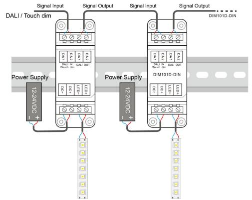
**Remark:** Only use open push button without indicator light. Maximum cable length between each Unit: 20 meters.
