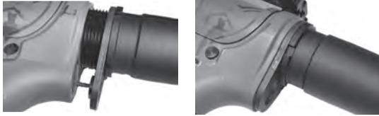
Carefully begin threading the tube into your lower receiver while ensuring the take-down detent spring remains straight as you thread the tube flush to the receiver. Use your castle nut wrench to torque the buffer tube to your receiver once it is flush.
