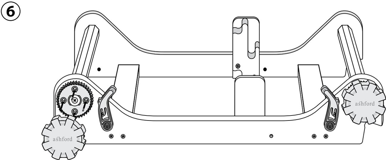
Locate the 4 pins on the handles into the 4 holes in the cogs. Then give the handles a sharp hit with your fist so they snap down tight onto the cogs.
