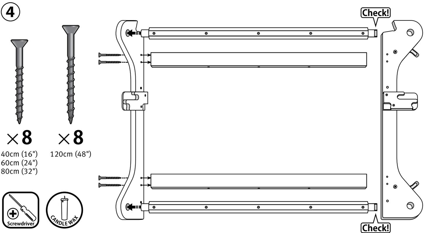
Attach the front and back rails to the left side with 38mm (1½") screws. Rub candle wax over both ends of the front and back roller, then insert the short end of the rollers into the holes in the left side.
