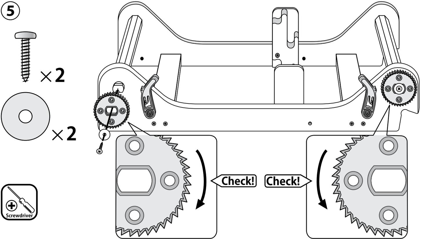
Place the cogs onto the ends of the rollers. Check the teeth engage the pawls. THEN secure with washers and 20mm ( $\frac{3}{4}$ " ) screws.
