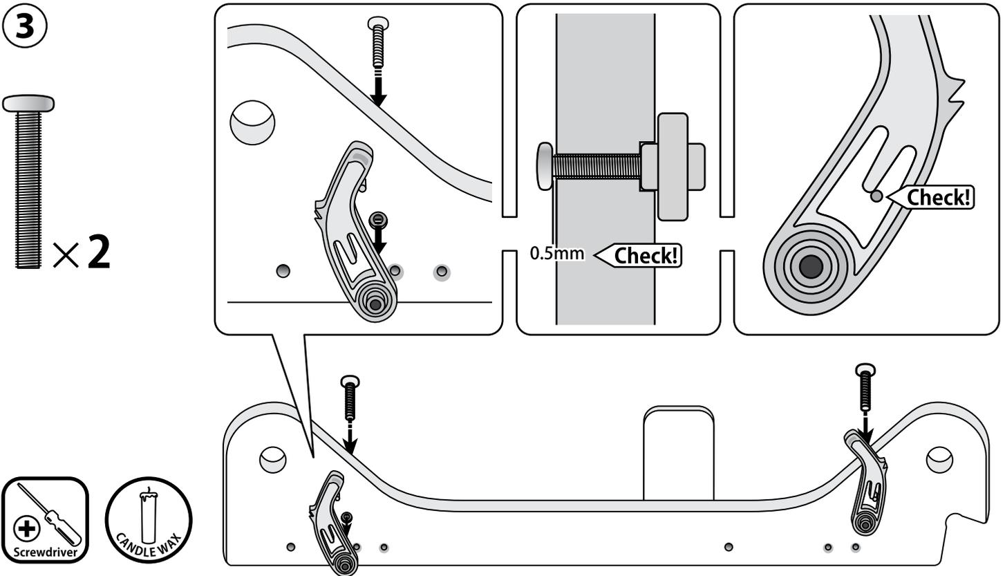
Attach the 2 pawls to the loom side from the inside with 30mm (1¼") bolts. NOTE the "clicker pin" fits into the gap in the pawl. Take care to ensure the "clicker pin" does not damage your table. Rub a little candle wax on the thread to make assembly easier. Leave 0.5mm (1/32") gap under the head of the bolt. DON'T over tighten. The pawl should move freely and "Click" as it snaps past the pin.
