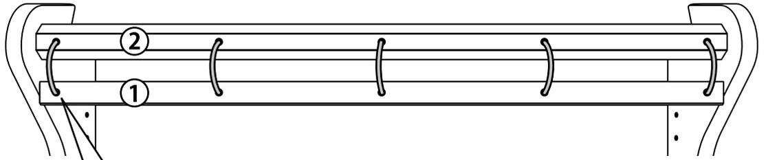
Connect the warp sticks to the roller with the warp stick ties. First push the arrow head through the warp stick. Then push the arrow head into the small hole in the roller and out the large hole as illustrated.
