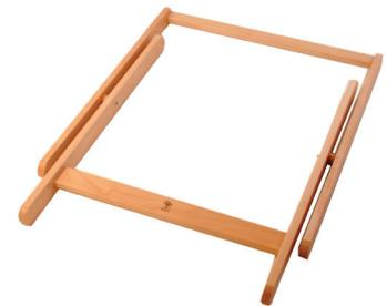
6. Position the legs with the wooden spacer between them, then insert the 2 x 75mm/3" bolts through from the inside. Tap the heads of the bolts into the wood and then secure with washers and nyloc nuts.
