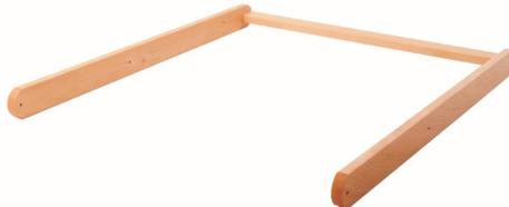
5. Assemble the other 2 legs and spacer rail with 2 x 50mm/2" screws each side.
