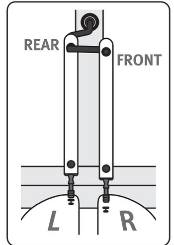
Note that the rear conrod attaches to the left treadle board and the front conrod attaches to the right treadle board.
