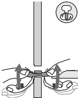
3 Slide it up into the small slot and turn it back a 1/4 turn until it clicks into place.
