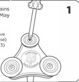
Carefully place new rubber foot onto pivoting head foot cavity.
