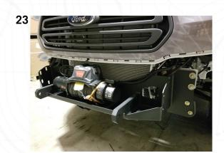
If equipped with the active cruise control sensor, remove sensor from factory bracket and install sensor into our new bracket. Install assembly onto the bumper making sure it's in the same orientation as it was from the factory. For the parking sensor cutouts on the bumper, either install the delete plugs (if not equipped with sensors) or install the supplied plastic sensor housings. Connect sensors into housings in the same location as the factory bumper.
