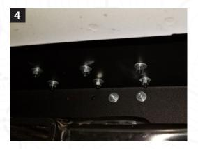
3. Using your mark from step one of removal, cut the plastic bumper cover at 4.75" down from top and reinstall the top portion using the OEM hardware and clips.
