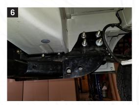
5. Using the supplied hardware from BW00-0040, bolt the bumper to mounting brackets. [**Team Lift**] Adjust the bumper to the desired height, and center it laterally on the van. **Pictures 7-8**
