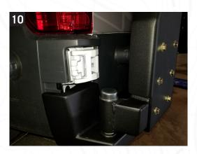
[The following set of instructions will result with the passenger side opening first, and the latch will be on the passenger side. If you prefer the driver door to open first, then install the latch setup on the opposite side.]
