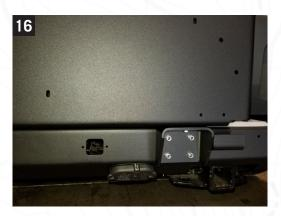
11. Install the lower latch rod support into the bottom two holes in the passenger side plate using the supplied countersink bolts in BW00-0020 sub 5 (one long, one short). Install the upper latch rod support into the 2 holes immediately above the overlap plate on the passenger side using the supplied counter sink bolts in BW00-0020 sub 5 (one long, one short). **Picture 17-18**
