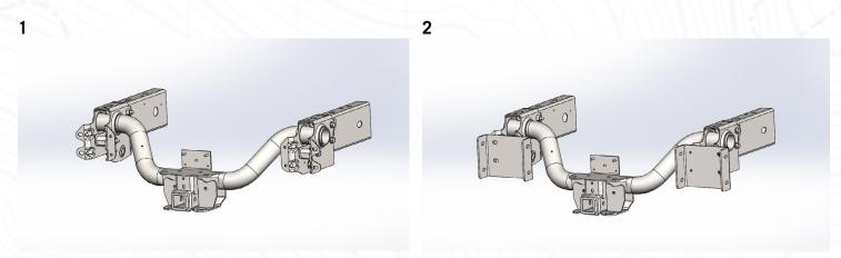
6. Using the supplied hardware, attach the 2nd set of brackets to the first set of brackets. See picture 3.
