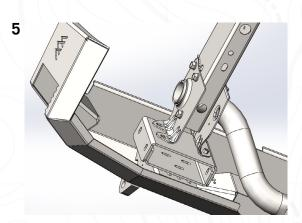
8. Adjust the bumper until desired fitment is achieved. Tighten the bolts to 80 ft-lbs. See picture 6 and 7.
