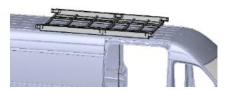
4) Raise the rear section onto the roof and similarly install the track bolts and connector bolts.
