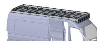
6) At this point, you may need to shift the entire rack forward or rearward for optimal fitment against the roof and around any vent fans. Once in the desired location, tighten the connector hardware, and finally, the rail/track hardware.
