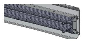
As with the other sections of the rack, raise the front section to the roof and secure it to the rails with the track bolts, and attach it to the center section with the 3/8" hardware.
