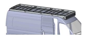
6) At this point, you may need to shift the entire rack forward or rearward for optimal fitment against the roof and around any vent fans. Once in the desired location, tighten the connector hardware, and finally, the rail/track hardware.
