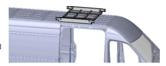
3) \*170" wheelbase only\* Install the 3rd section: While still on the ground, install the rear connector brackets using more of the 3/8" hardware. Raise this section onto the roof. Install the track bolts, then connect this section to the section from step 2.
