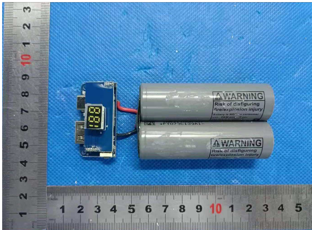
Picture 4. Inner view-1 of battery
