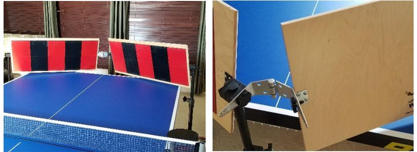
In this configuration you may prefer to attach the double bouncer bracket to the boards using the middle holes in the bracket instead of the end holes as this produces a smaller gap between the boards.
