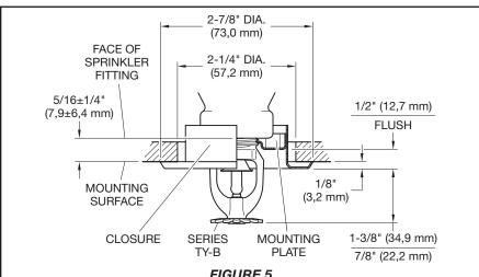
FIGURE 5 SERIES TY-B RECESSED PENDENT SPRINKLER ASSEMBLY (TY325) WITH TWO-PIECE 1/2 INCH TOTAL ADJUSTMENT STYLE 20 RECESSED ESCUTCHEON
