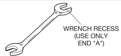
FIGURE 3 W-TYPE 6 SPRINKLER WRENCH
