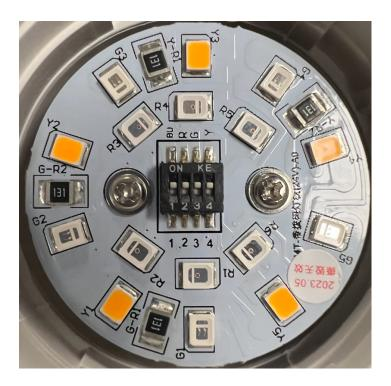
To access the dip switches, twist off the clear and white cover.
