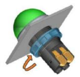
3 0.4-0.6N.m Tighten the nut counterclockwise
