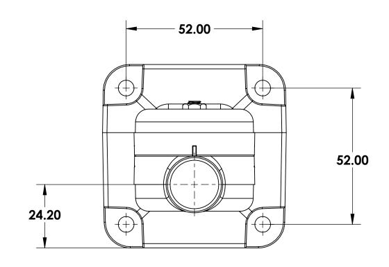
Swivel Rotates 90 Degrees Comes in Black or White Plastic Works with MC50 and SL60 Stack-Lights
