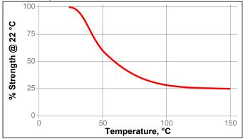
Cured for 5days @ 22 °C Lap Shear Strength, : Steel
