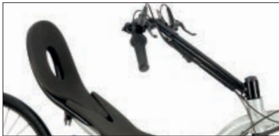
Alternatives for the cockpit: The tiller steering handlebars combine a relaxed arm position with good aerodynamics. The hands lie loosely in front of the chest.
