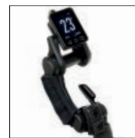
Right: On the under seat-steered Streetmachine Gte , the "Top View" mounting at the handlebar end can be used to bring the display closer to your field of vision, but slightly reduces the space available to mount the bike. Alternatively, it can be mounted next to the handlebar handle (picture bottom left).
