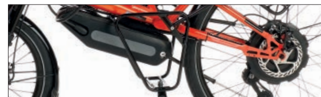
Top: The battery is ideally placed in the middle of the bike under the seat with a low centre of gravity. All HP VELOTECHNIK recumbents with above seat steering offer space for this, the Streetmachine Gte also with underseat steering. The lockable battery can be easily removed for charging.
