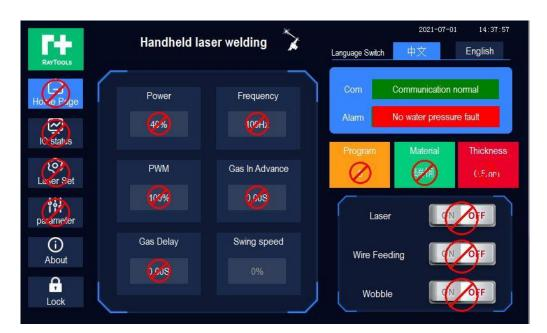
Lock: To lock the screen and cannot operate HMI. It mainly prevents other people from touching the screen by mistake when the operator is operating, causing the laser beam turned off while welding or the laser beam is emitted when the operator is commissioning, so as to ensure the safety of the operator.
