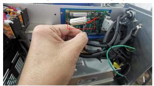
If the voltage is about 4.5V, remove the beam combiner inside the laser path and replace it with a wooden board.
