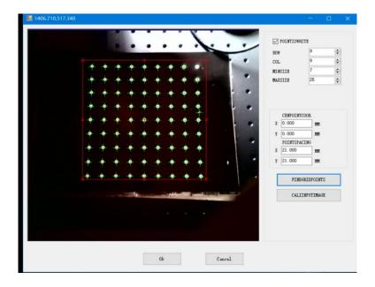
6. Copy the saved calibration file into the Ezcad2.14.11(20210302) - LitePro folder (a prompt will appear to overwrite, select overwrite), open the Ezcad2 program, and mark a pattern.
