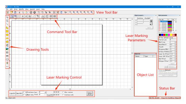
Cloudray LiteMarker marking machine is controlled by the included EZCad2 software, which must be installed on a compatible computer to direct the laser. See its separate instruction for full details on its components and use. Some features which are particularly important to note include the following parameters and controls:
