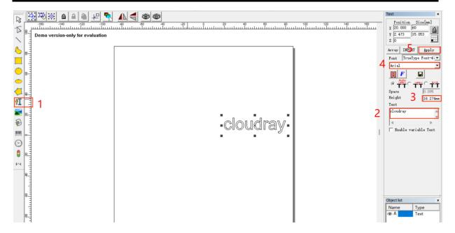
2. Adjust the text direction as required.
