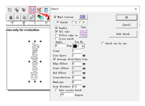
5. Menu bar—Laser—Rotate Text Mark—Set parameters
