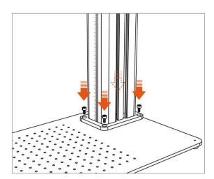
**Step 2.** Install the light path onto the lifting column using the provided screws. Tighten the four screws with the Allen key.
