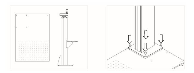
**Step 2.** Adjust the nut at the bottom of the light path to an appropriate position. Install the light path onto the lifting column using the provided screws. Tighten the four screws with the Allen key.
