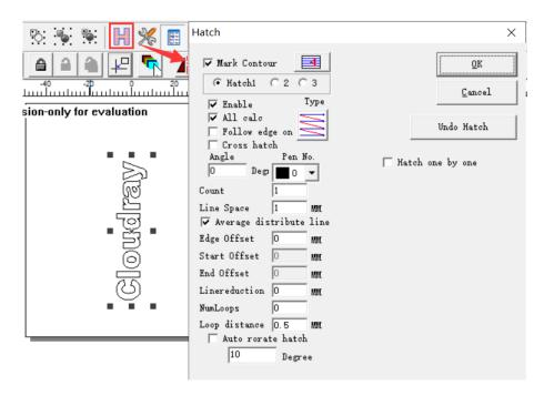
5. Menu bar—Laser—Rotate Text Mark—Set parameters
