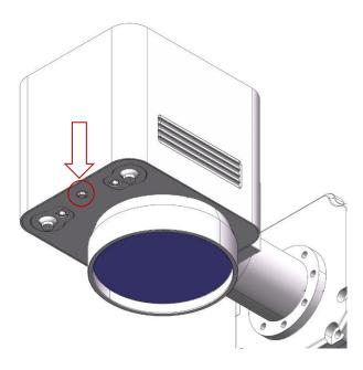
Step 6. Turn the focus wheel to adjust the two red dots to coincide to achieve focus.
