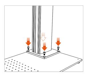
**Step 2.** Adjust the nut at the bottom of the light path to an appropriate position. Install the light path onto the lifting column using the provided screws. Tighten the four screws with the Allen key.
