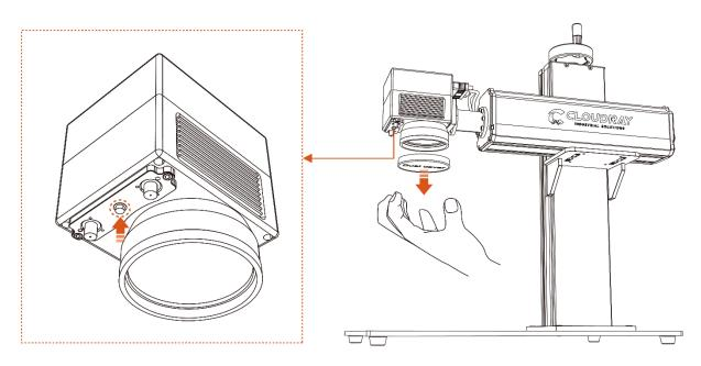
**Step 6.** Turn the focus wheel to adjust the two red dots to coincide to achieve focus.
