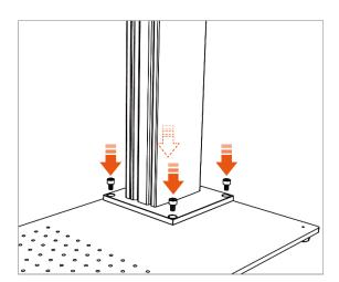
**Step 2.** Adjust the nut at the bottom of the light path to an appropriate position. Install the light path onto the lifting column using the provided screws. Tighten the four screws with the Allen key.
