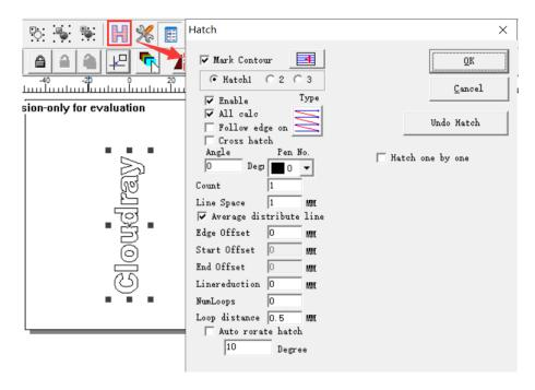
5. Menu bar—Laser—Rotate Text Mark—Set parameters
