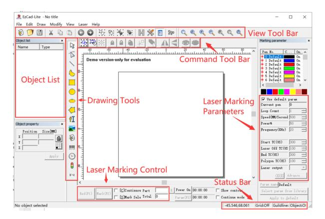
Cloudray LiteMarker marking machine is controlled by the included EZCad2 Lite software, which must be installed on a compatible computer to direct the laser. See its separate instruction for full details on its components and use. Some features which are particularly important to note include the following parameters and controls:
