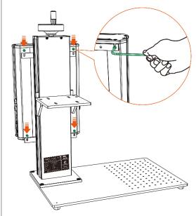
**Step 3.** Adjust the nut at the bottom of the light path to an appropriate position. Install the light path onto the lifting column using the provided screws. Tighten the four screws with the Allen key.
