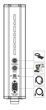
**Step 5.** Plug in the U disk (software, driver, electronic manual), and connect the USB cable to the PC.
