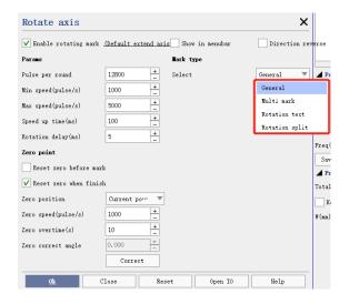
**Pluse per round**— The number of pulses required for the extension axis motor to rotate one round. We can calculate the number of pulses per revolution X required by the software through the following formula:  $X=(360/N)^* n$ , where X represents the number of pulses per revolution, N represents the step angle of the motor we use, and n represents Is the subdivision number set by the driver.
