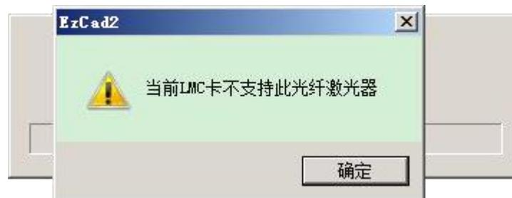
Failure reason: the control card is not connected to the computer or not powered;
