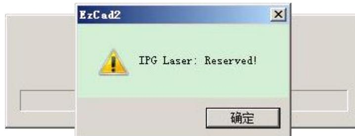
Fault reason: the laser is not connected or not powered;
