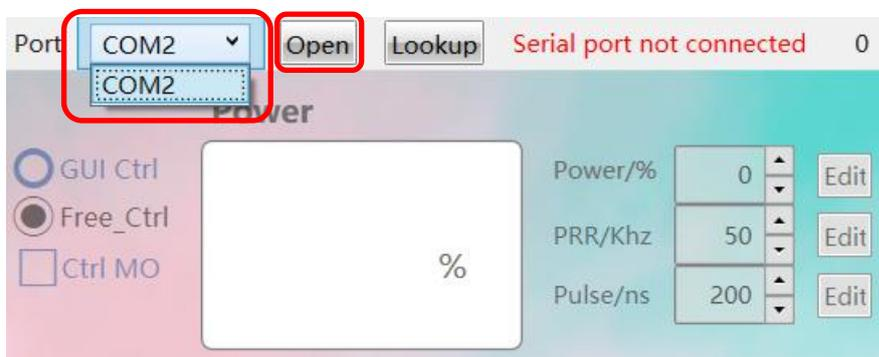
**Figure 1 The selection of GUI Serial Port connection**
