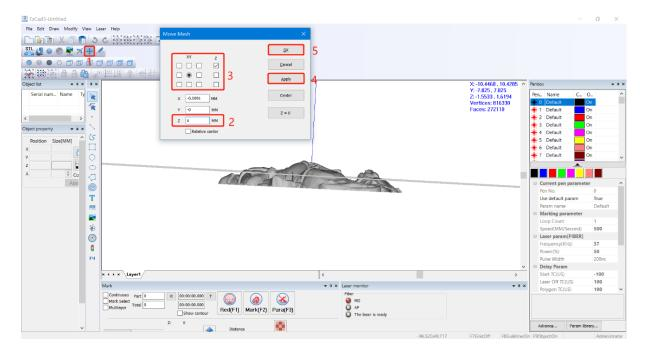
After adjustment, the file is moved below the surface, as shown in the image below.
