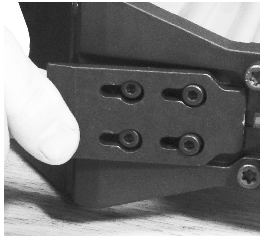
Step 2. Slide gage plate off.
