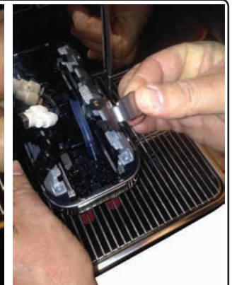
Push the metal lock to the front and remove it.
