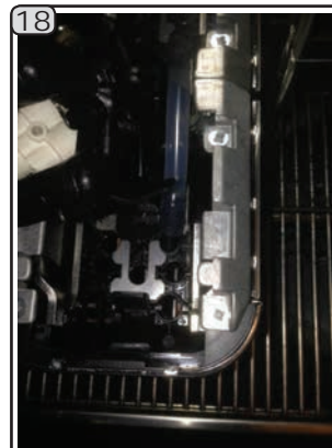
Push the metal lock to the front and remove it.
