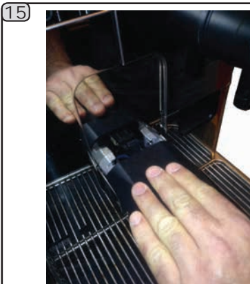
Remove the cover from the dispensing nozzle.
