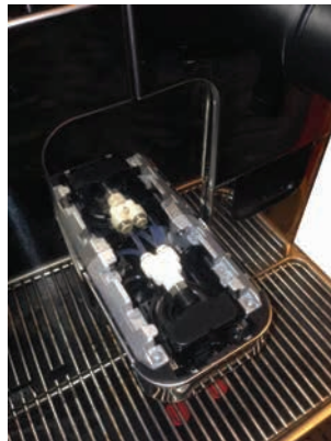
Remove the cover from the dispensing nozzle.
