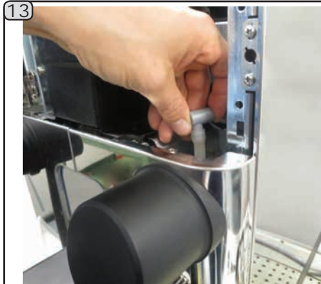
Remove elbow from the silicone pipe.
