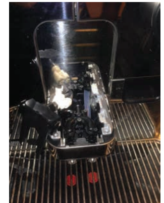
Push on both sides and move the coffee spout as shown above.
