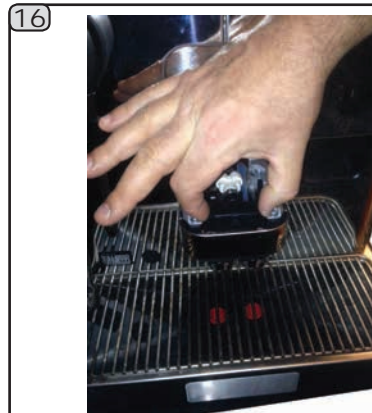
Push on both sides and move the coffee spout as shown above.
