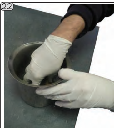
22 Put a sponge in the solution and then clean the mixer fixed part.
