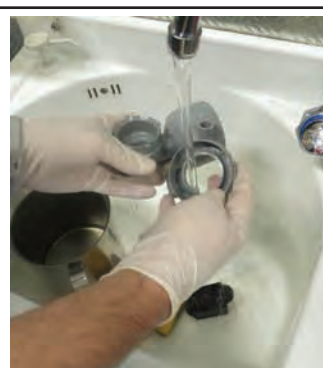
25 Rinse all parts (fixed part too) with cold water accurately.
