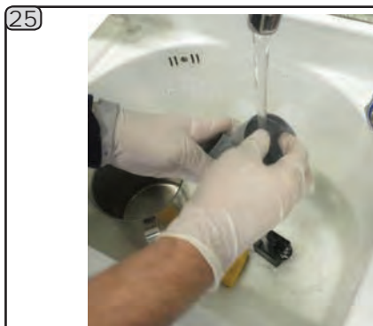
25 Rinse all parts (fixed part too) with cold water accurately.
