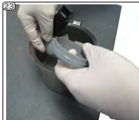
23 Put all the removed mixed parts (except the soluble hopper) in the solution, then clean them accurately with a sponge.
