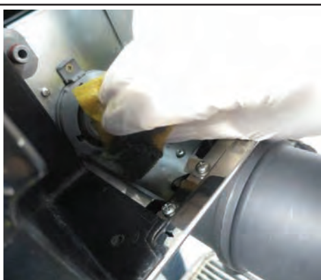
22 Put a sponge in the solution and then clean the mixer fixed part.
