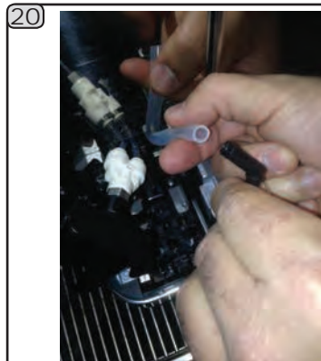
20 Remove elbow from silicone pipe, then clean pipe with the brush.
