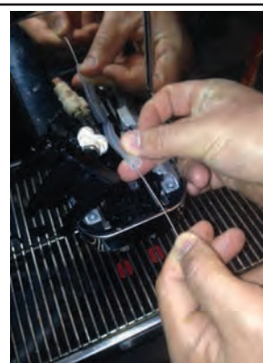
20 Remove elbow from silicone pipe, then clean pipe with the brush.
