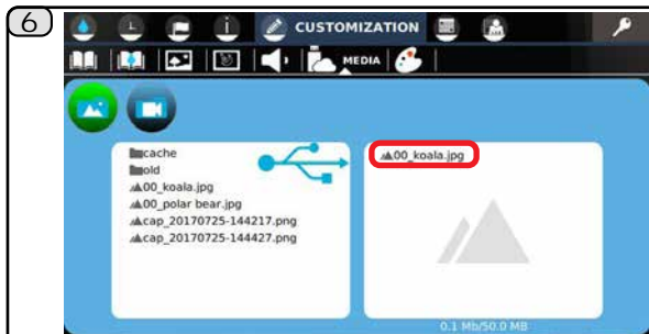
When copying is complete, the selected files will appear in the machine memory.
