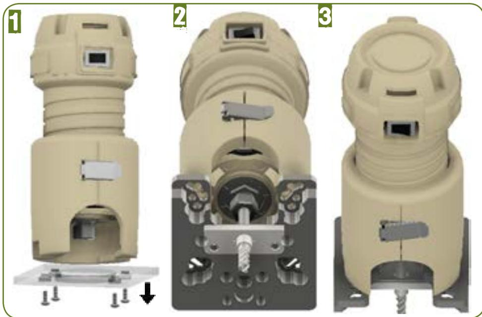
Reuse the router's screws to loosely attach the router attachment plate. If the router has tapered screws, replace them with screws that have a flat inner face. The metric M4-0.7 pan head screws provided with your jig will fit most compact routers. Make sure the thread pitch matches that of the router before attempting to use the screws. Do not tighten the screws at this time. **Do not use screws which have a conical tapering inner face with the router attachment plate.**
