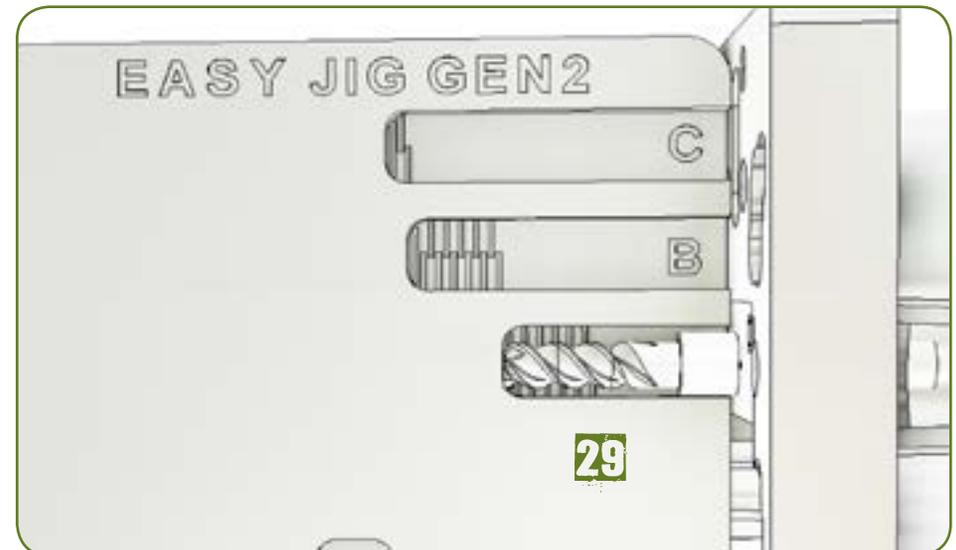
After milling the full depth for depth gauge “A”, insert the long 1/4” quick release pin into the main jig plate to prevent further milling to the rear shelf (Fig. 20). The pin may already be inserted into the jig plate if you have been milling only the main trigger pocket area for a Gen 2 lower.
