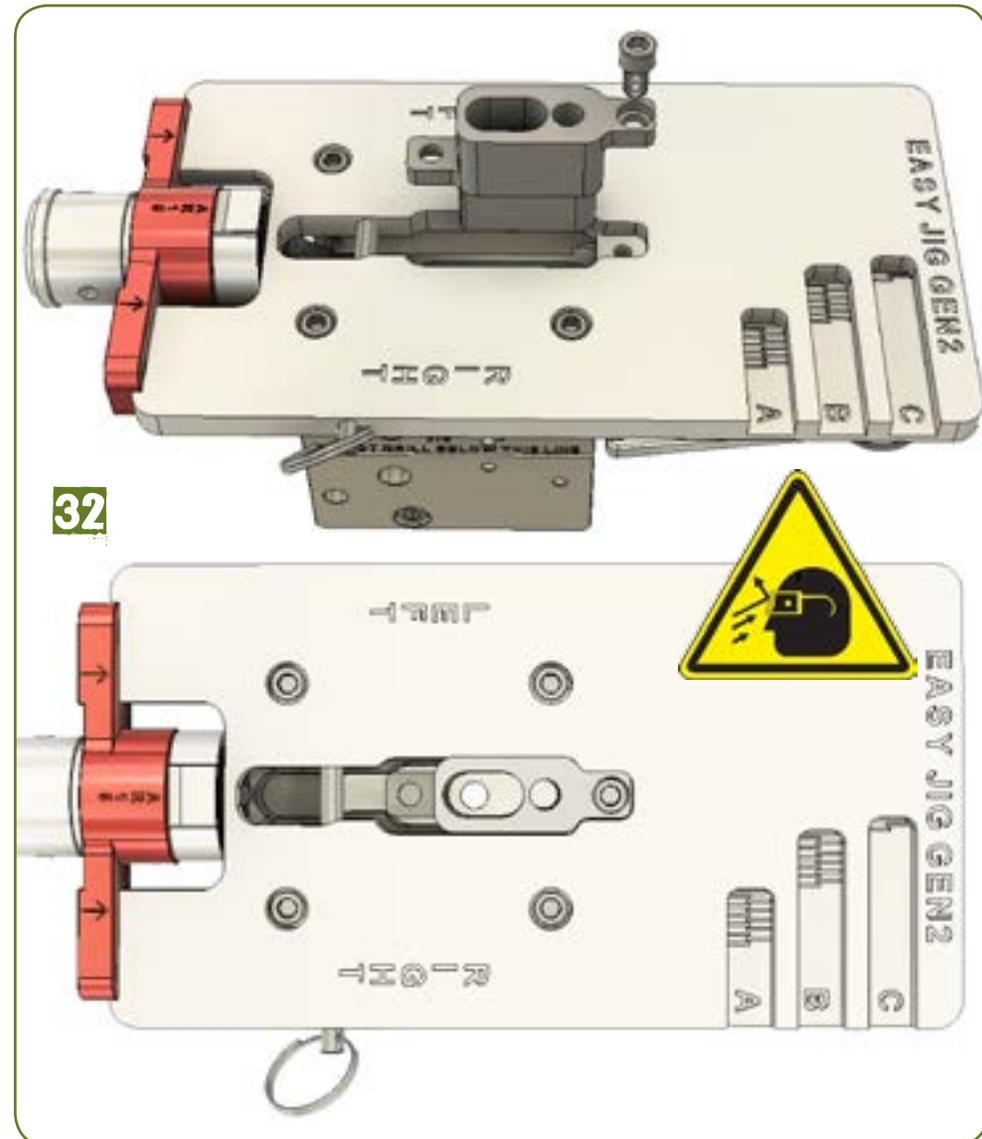
Press the router attachment plate flush against the right side of the jig with the bushing fully inserted into slot "C". Adjust the router depth so the tip of the end mill is centered on top of the first hash mark (Fig. 33). Insert the bushing and end mill into the oval slot of the trigger template and through the 21/64" pilot hole (Fig. 34). Make sure the router attachment plate is flush on the main jig plate to confirm the end mill is inside the pilot hole (Fig. 36).
