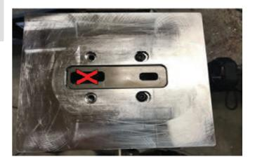
The larger slot over the magazine well is not used. Adjust the router depth setting so the end mill is slightly inside the drilled out trigger slot pilot hole. With the end mill centered in the hole, turn on the router while keeping a firm grip on the router. Mill back and forth in a clockwise motion. Turn off the router and increase the depth by 1/6 to 1/4 notch and repeat the process. Continue until the trigger slot is fully milled out.
