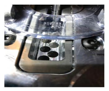
Maintain a firm grip on the router when turning it on. For your first cutting pass, only focus on removing material between the holes using a zig-zag pattern until all the holes are connected. Take your time and go slow. This first pass will take you 1-2 minutes. Do not change the depth of the end-mill yet.
