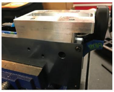
Then stack the Trigger Pocket Template #05 so that the smaller end and the hole on the template is toward the buffer tube hole, and the raised lip on the template is facing up.
