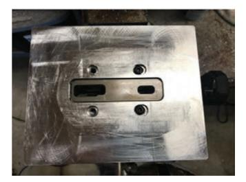
Secure the Router Base Support Plate #07 on top of the template using only the 2 short Trigger Milling Bolts #10. Only use 2 bolts to attach the template and base plate. Insert the screws into the 2 holes on the base plate closest to the buffer tube, using the 2 screw holes on the jig side plates furthest from the buffer tube. The smaller trigger slot should be located closest to the buffer tube.
