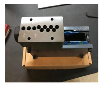
Tighten the top bolts in an "X" pattern to ensure you have your jig walls parallel and spaced apart correctly.
