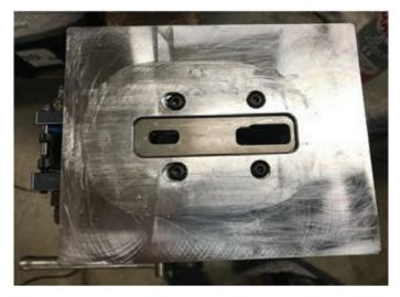
Tighten the bolts to the jig walls in an alternating ("X" shape) pattern. Secure the assembled jig in the vise with the buffer tube hole facing away from you.
