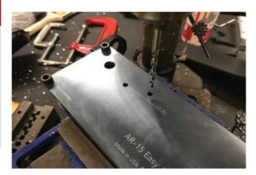
Next, install the 3/8° Drill Bit #13 and drill out the safety selector hole on the right side.
