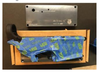
**PROCEED:** Attach side plates #01 and #02 to lower receiver using the Jig Wall Bolts #08. The bolts will go through side plate #01 (Right Jig Wall) and thread into side plate #02 (Left Jig Wall). The top bolts will be going through the takedown pin holes in your lower receiver.
