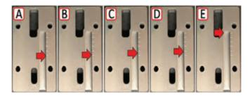
Each image in A-D shows a 1/4 notch or hash mark incremental move. For the final pass, set depth to very top edge of gauge as shown in E.)
