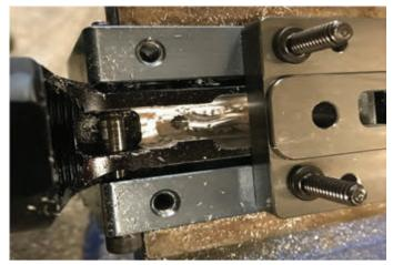
Place the Trigger Pocket Template #05 on the jig with the depth gauge facing down and the trigger pilot hole facing towards the buffer tube. Attach the Trigger Pocket Template #05 to the jig side plates, inserting only the 2 short Trigger Milling Bolts #10 into the two jig wall screw holes furthest away from the buffer tube to secure the template. Secure the Jig into the vise. Using the 19/64" Drill Bit #15, slowly drill the pilot hole.
