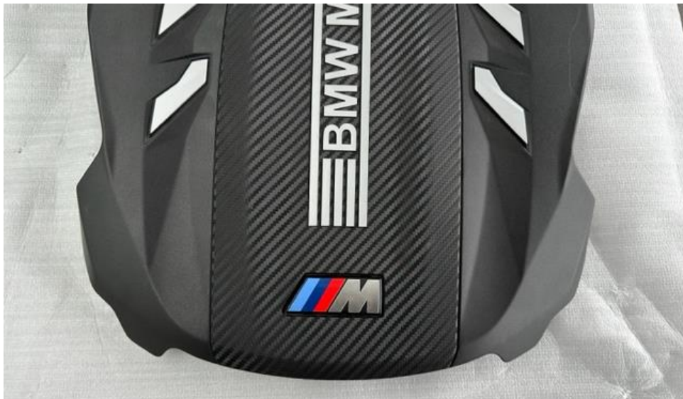
27. Remove the M Badge – these are tabs on the back which can be carefully folded back to allow the badge to be removed.
