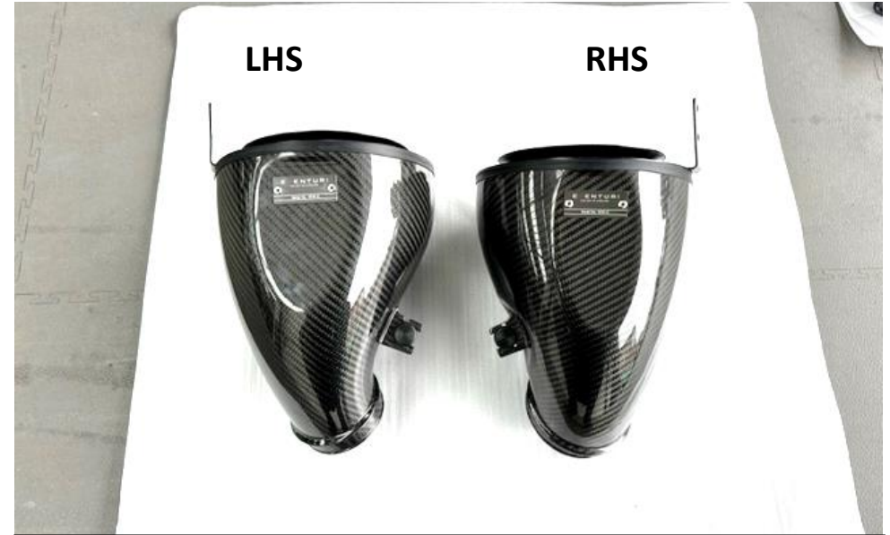
14. Identify the LHS and RHS Filter Housings.
