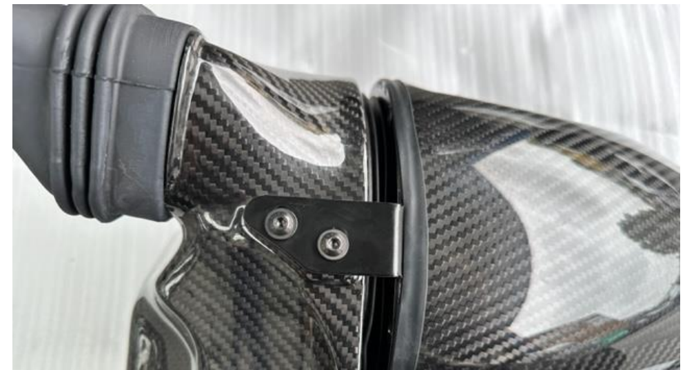
16. Use 2 of the supplied M5 screws and locate them into the bracket as shown to keep the filter housing and duct together. Don't tighten them yet.
