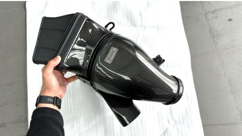
15. Place the LHS Housing inside the RHS Duct. The metal filter cowl should go into the duct so the rubber seal should be pressed against the flat part of the filter cowl.
