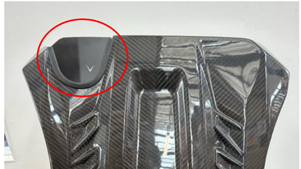
32. If you have the reservoir as shown previously, remove this blanking plate and the rubber trim from the carbon engine cover. The can just be pulled out.
