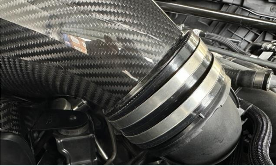
21. Push the intake down into the grommets and into the silicon. Once fully located, pull the silicon coupler upwards to meet the flange around the carbon housing.
