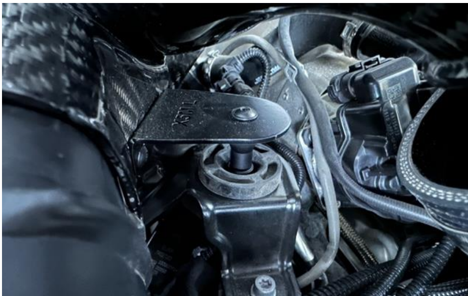
19. Line up the mounts on the intake with the grommets – there are 3 in total.
