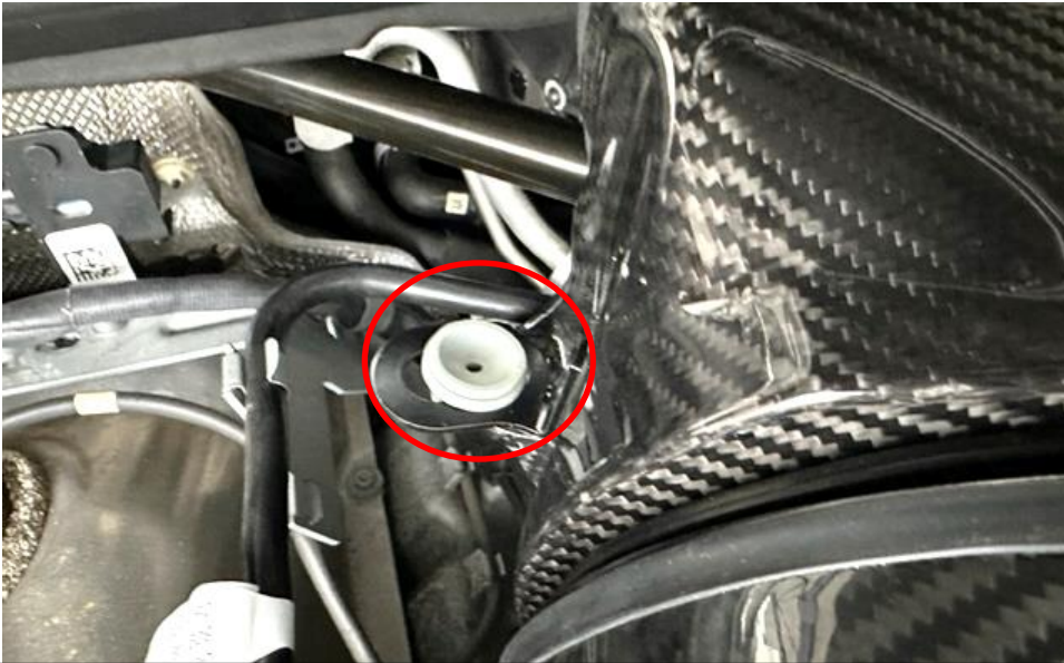
29. Push the rubber grommets from the stock airboxes onto the brackets on the carbon ducts.
