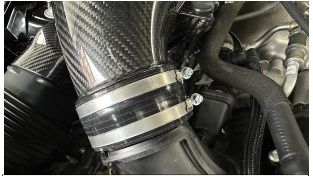
22. Tighten the hose clamps. DO NOT overtighten around the carbon. It only needs to be hand tight.
