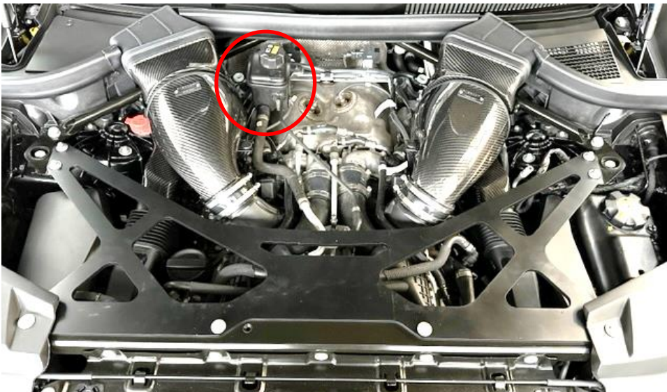
31. Reinstall the strut brace. If you have this reservoir in this position as circled then go to the next step. If your reservoir is not in this position, go to step 33.
