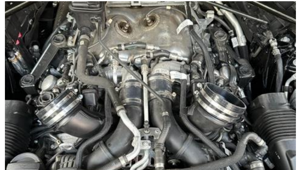
8. Install the supplied silicon couplers to the turbo inlets. There are 2 sizes provided. The larger one goes onto the Right inlet.
