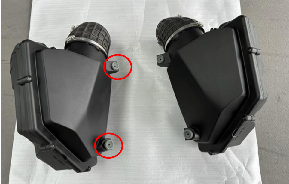
25. Remove only 2 of the grommets for the engine cover from the stock airboxes.
