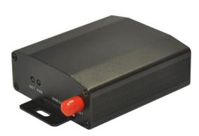
The W-Link WL-M303-6 is a robust industrial LTE USB modem that provides SMS and dial up function in GSM, Edge and 3G networks. The modem has a wide operating temperature range and mounting provision making it ideal for most industrial applications. Configuration and control can also be done with AT commands. Up to 100Mbps download and 50Mbps upload speeds. Supports USB2.0
