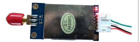
When RF1276-868 is transceiving data, the LED of the module will show BLUE
