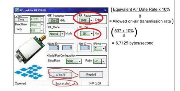
If the transmitting period is 500ms, we transmit the data packet of 'www.appconwireless thank you for choosing our module' (total 50bytes). We send the total data up to 850bytes
