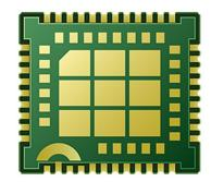
The SIM7080 series is the LPWA module which supports wireless communication modes of CatM/-Cat-NB. This series adopts LCC and LGA form factor and has a compact size of 17.6mm\*15.7mm which makes it ideal for compact products design.
