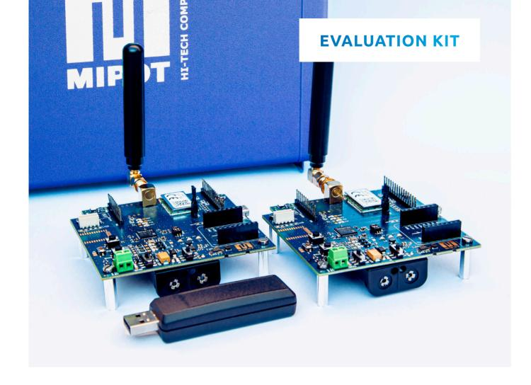
All features of the Wireless M-Bus and LoRa® modules can be tested with our dedicated Evaluation Kit. The board provides easy access to module pin-out, power supply pins and SMA antenna connector. Usage flexibility is given by several power supply modes.
