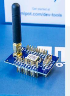
Equipped with 3 pin strip connectors, the kit allows easy interfacing with all LGA pads on the MiP module via jump wires or a perfboard. The developer can use the Devkit both in **host-based mode**, connecting his own controller to the board, or **as a stand-alone product** exploiting the full potential of the MiP Series modules. The package includes a development board with SMA connector, a **monopole antenna** for 868 MHz and 915 MHz frequency bands and a reference sheet.
