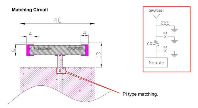
Between antenna and module need a pi type matching circuit.
