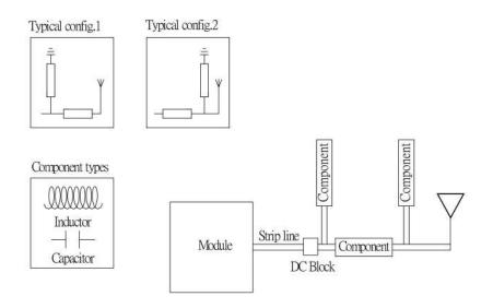
The matching network has to be individually designed using one, two or three components.
