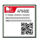
A7682E is the LTE Cat 1 module that supports wireless communication modes of LTE-FDD/GSM/GPRS/EDGE. It supports maximum 10Mbps downlink rate and 5Mbps uplink rate. A7682E adopts LCC+LGA form factor and is compatible with SIM800C, SIM868series (GSM/GPRS modules), which enables smooth migration from 2G products to LTE products, and greatly facilitates more compatible product design for the customer needs.
