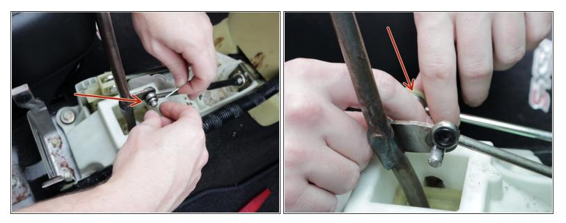
Disconnect both shifter cables. You may need to use pliers to get the OEM cotter pin out. Shown is the Hybrid Racing shifter cable inserts, (HYB-SCB-01-05)
