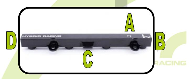
**Port A:** Optional to run a fuel pressure gauge here,. If you are not installing a gauge, install the stainless steel NPT plug here. Be sure to place fuel-safe sealant on the threads whether you are running a gauge or the plug.
