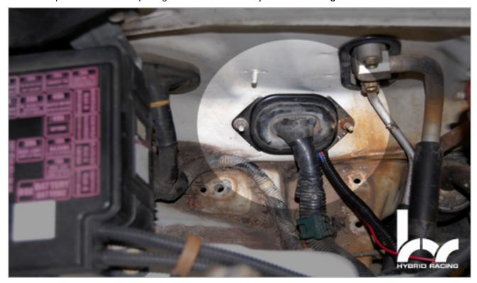
4. Route the **K series engine harness** through the firewall on the passenger side utilizing the factory grommet.
