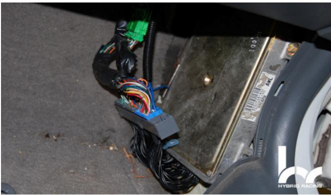
3. Remove the factory engine harness from the engine bay and under the dash. There will be 2 10mm bolts under the battery tray holding the harness in place. Remove this plate/grommet to reuse with your **K series engine harness**.
