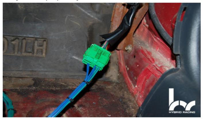
7. Connect the C302 from your Hybrid Racing harness to the connector on the K series engine harness.
