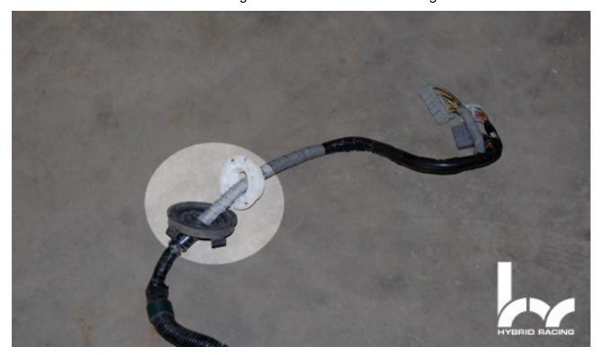
5. Run the hybrid racing harness along the inside of the floor, near the firewall. You should have all of the connectors in one area.
